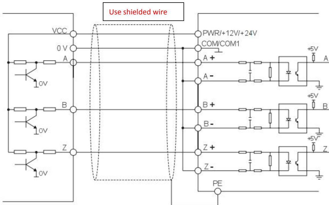
**Note:** A-, B-, Z- of the PG card are short-circuited with COM, and the encoder VCC, 0V, A, B, and Z are connected to the PWR, COM, A+, B+, Z+ of the PG card correspondingly.
