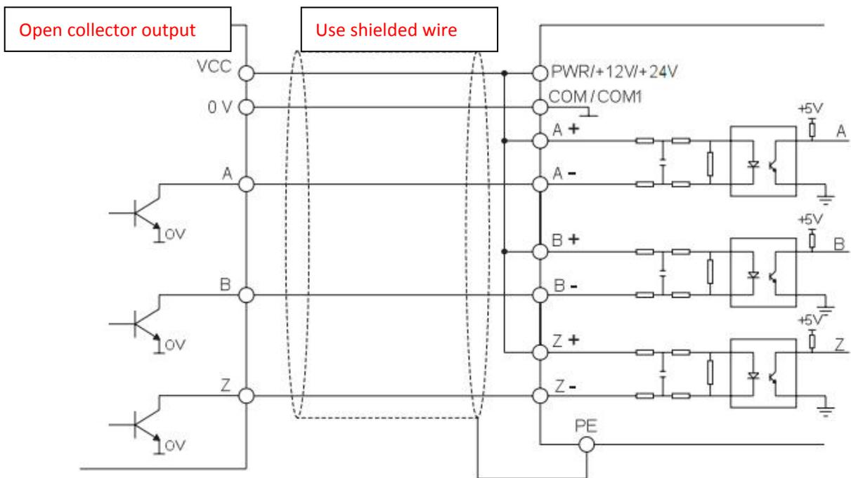
**Note:** A+, B+, Z+ of the PG card is short-circuited with PWR, and the encoder VCC, 0V, A, B, and Z are connected to the PWR, COM, A-, B-, Z- of the PG card correspondingly..
