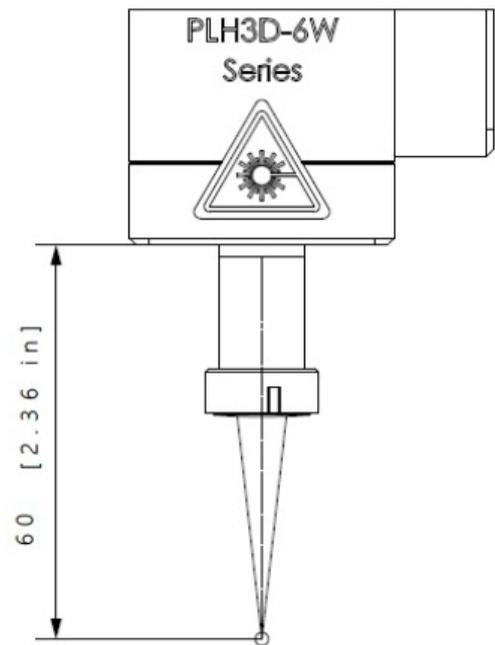
the Beam Cone Shape of the PLH3D-6W-µSpot Laser Head
