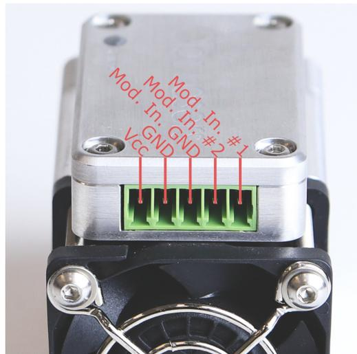
Cable pinout for PLH3D-6W-Hobby and other pigtailed PLH3D-6W-Series engraving laser heads (sold before 01.10.2020)
