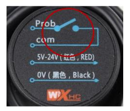
When RF LED is not going on when Prob is used, check connection to receiver.
