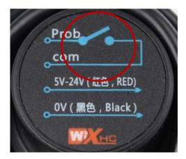
When RF LED is not lighting when Prob is used, check connection to receiver.
