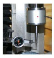
Mount the Econo-Probe in your machine and setup an indicator as shown above. It is critical to achieving accurate alignment that the indicator be held firmly in place. Place the point of the indicator as close to the center of the spherical tip as possible (in other words, "along the equator"). Have a note pad handy.
