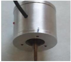
In order to make the balance of this procedure easier, mark, on the outside housing, the position of each adjustment screw (see photo above). Use whatever type marking you want, including a scribe if you wish the marks to be permanent for future alignments. It may also be helpful to number the adjustment screws for easier reference through the balance of the procedure.
